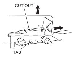
Lift the tray clear of the guide rail and out of the merchandiser.
