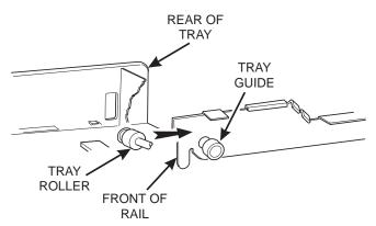
4. Hold the tray up while pushing it toward the rear. Stop when the tab on the tray aligns with the opening in the tray guide.
